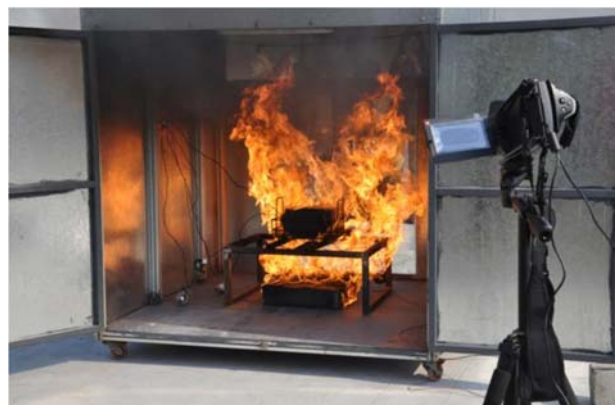
外火引燃实验 The test of ignition
