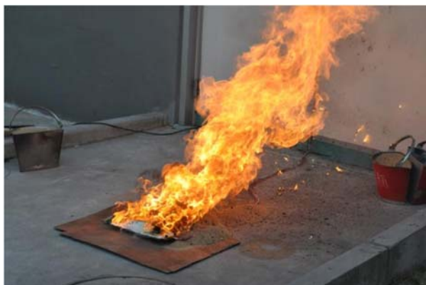
过充着火实验 The fire test of overcharge
