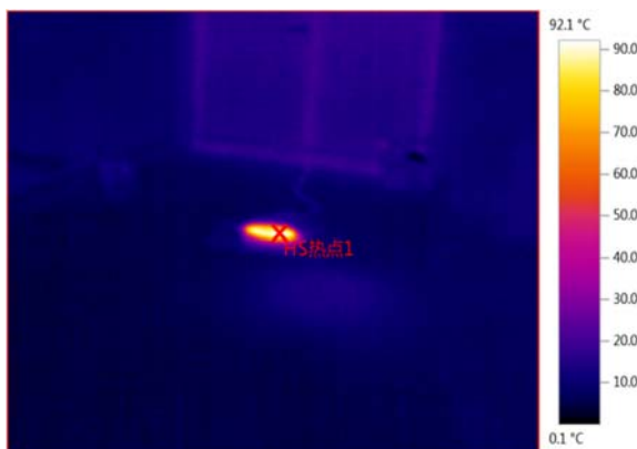
着火临界状态 Critical state of Ignition
